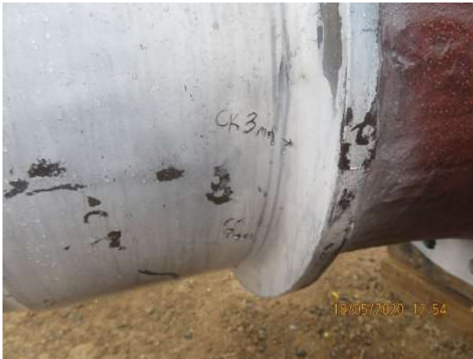
PHOTOGRAPH NO. 8 - 3mm crack detected
