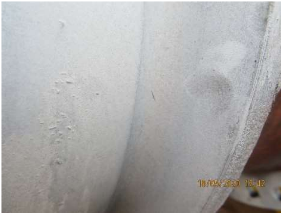
PHOTOGRAPH NO. 6 - 5mm crack detected
