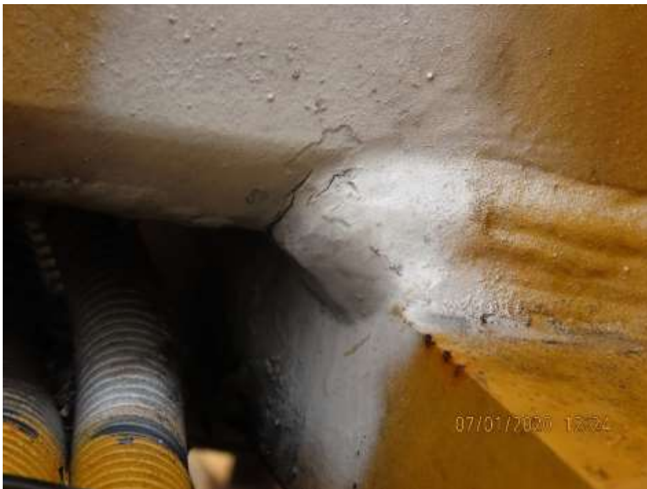
PHOTOGRAPH NO. 16 - Caterpillar 6060 excavator superstructure - 40mm crack detected.
