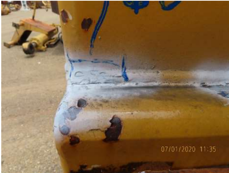
PHOTOGRAPH NO. 14 - Caterpillar 6060 excavator superstructure - 50mm crack detected.
