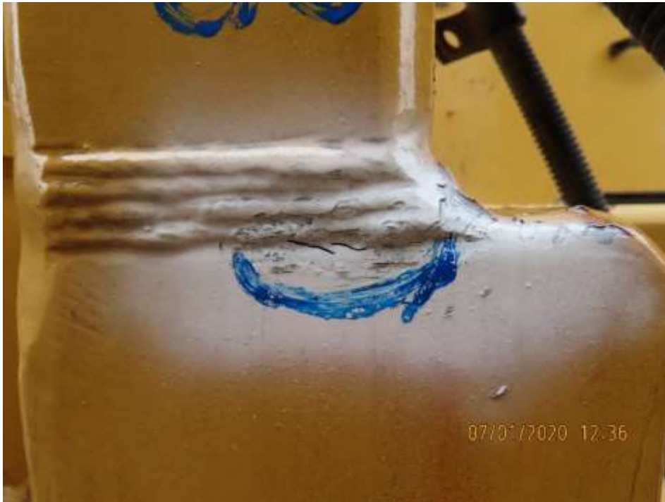
PHOTOGRAPH NO. 16 - Caterpillar 6060 excavator superstructure - 40mm crack detected.
