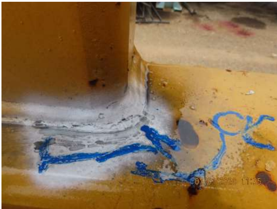
PHOTOGRAPH NO. 14 - Caterpillar 6060 excavator superstructure - 50mm crack detected.
