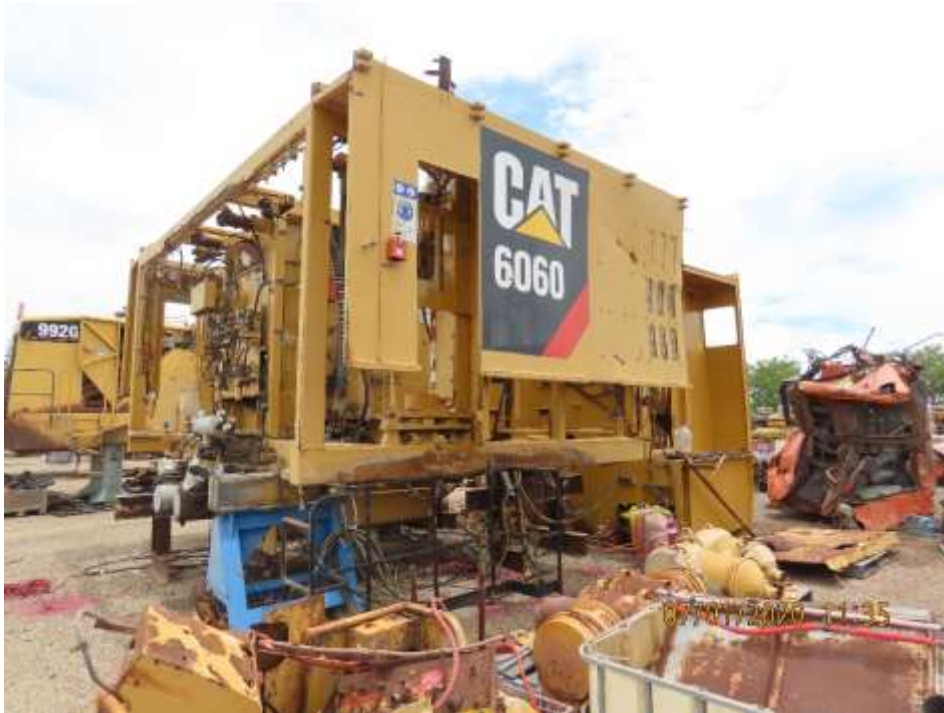
PHOTOGRAPH NO. 4 - Caterpillar 6060 excavator superstructure - corrosion detected on right hand side rail.
