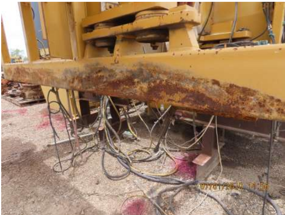
PHOTOGRAPH NO. 4 - Caterpillar 6060 excavator superstructure - corrosion detected on right hand side rail.
