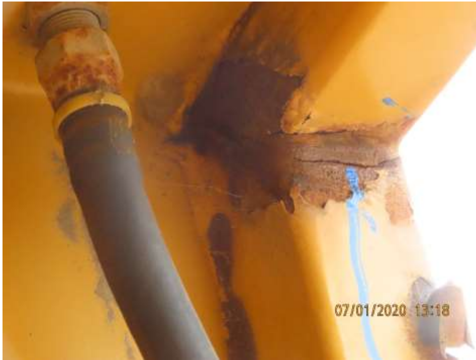
PHOTOGRAPH NO. 22 - Caterpillar 6060 excavator superstructure - crack detected on roof support.
