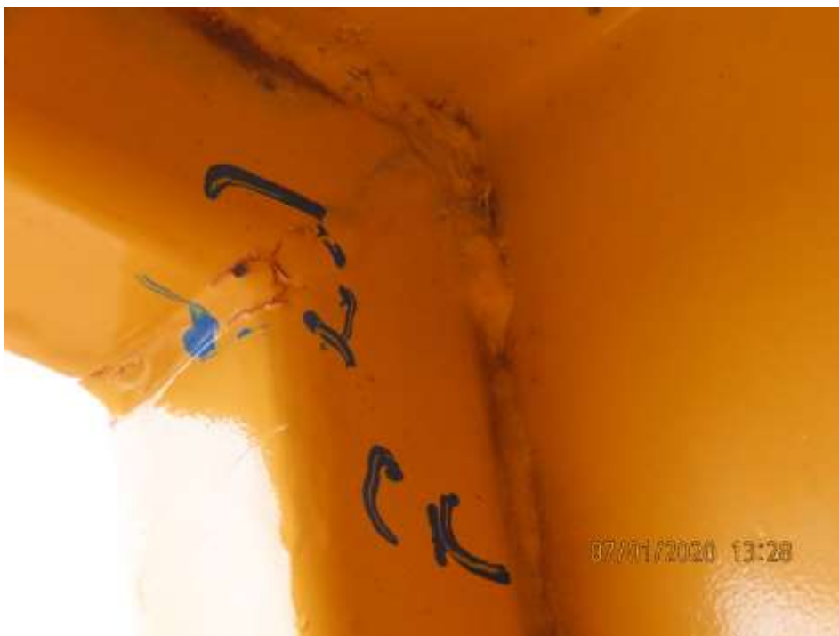
PHOTOGRAPH NO. 24 - Caterpillar 6060 excavator superstructure - crack detected on roof support.
