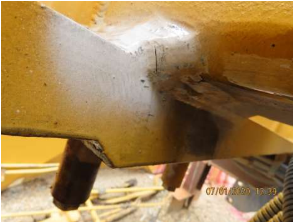
PHOTOGRAPH NO. 18 - Caterpillar 6060 excavator superstructure 200mm, 186mm, 152mm, 101mm, 93mm & 72mm cracks detected.
