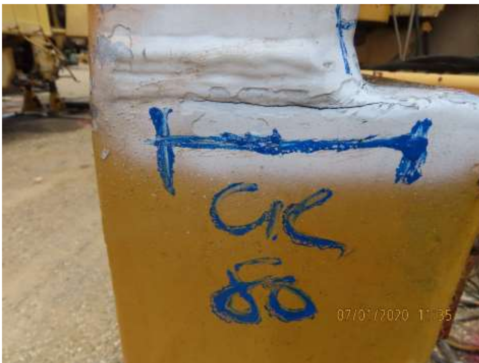
PHOTOGRAPH NO. 12 - Caterpillar 6060 excavator superstructure - 80mm crack detected.
