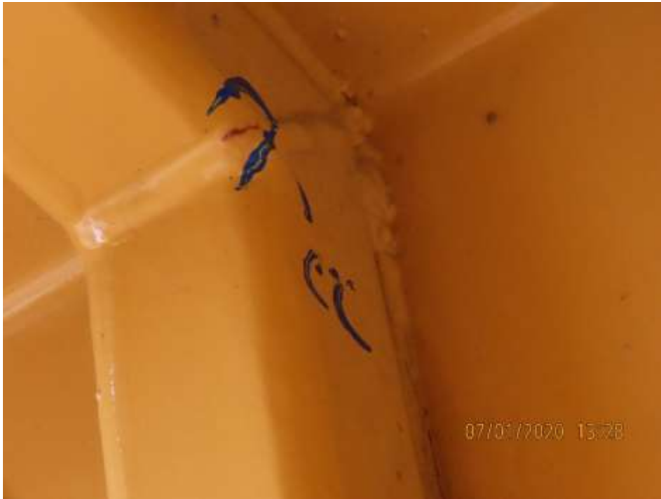
PHOTOGRAPH NO. 24 - Caterpillar 6060 excavator superstructure - crack detected on roof support.
