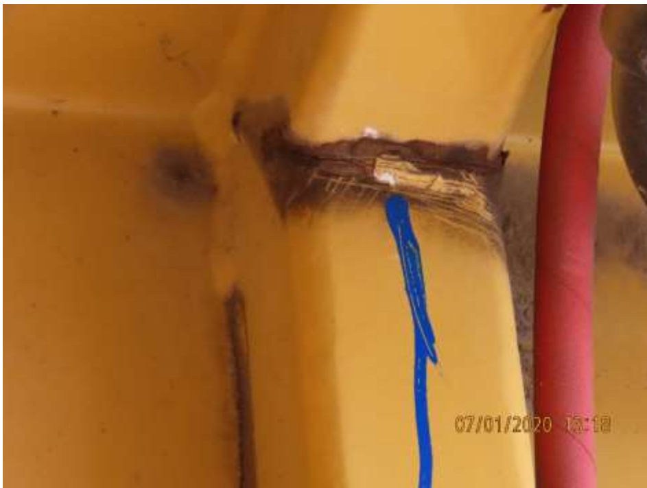
PHOTOGRAPH NO. 20 - Caterpillar 6060 excavator superstructure - crack detected on roof support.
