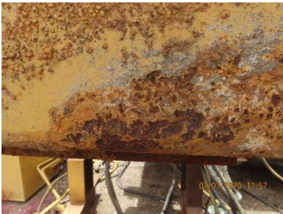
PHOTOGRAPH NO. 6 - Caterpillar 6060 excavator superstructure - corrosion detected on right hand side rail.
