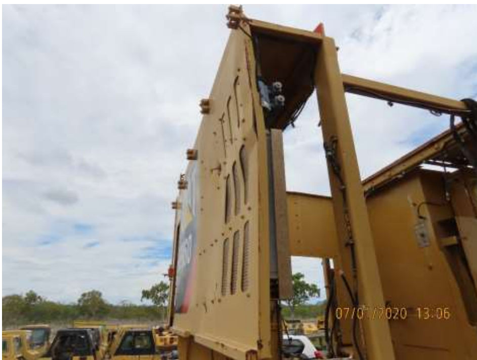
PHOTOGRAPH NO. 10 - Caterpillar 6060 excavator superstructure - mechanical damage detected on left hand side panel
