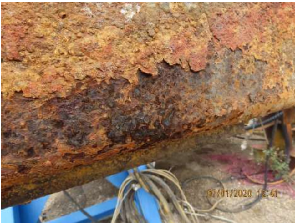
PHOTOGRAPH NO. 8 - Caterpillar 6060 excavator superstructure - corrosion detected on left hand side rail.
