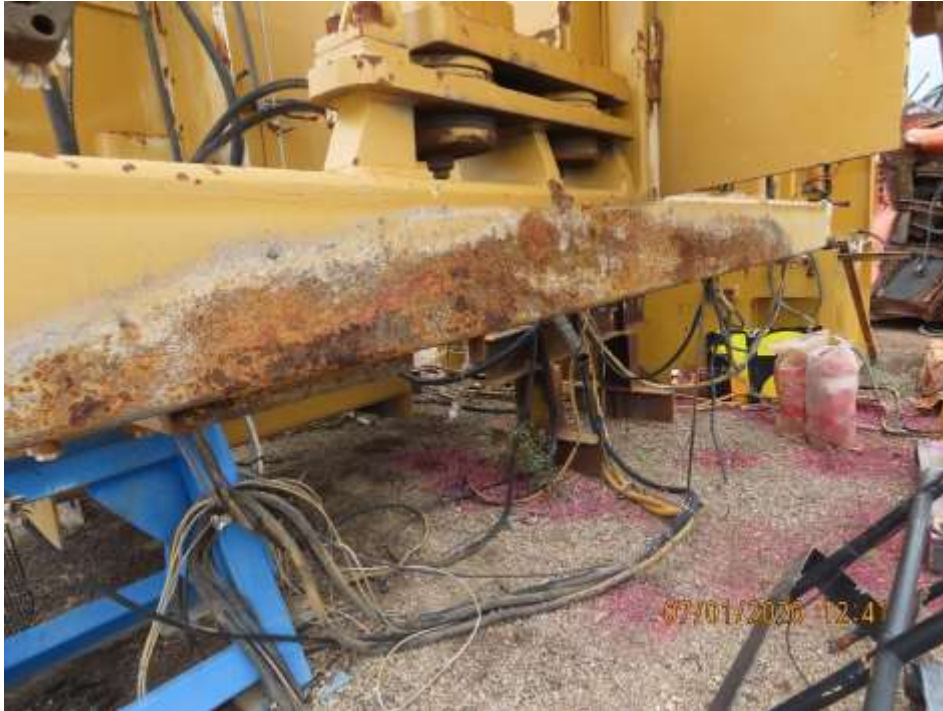
PHOTOGRAPH NO. 8 - Caterpillar 6060 excavator superstructure - corrosion detected on left hand side rail.
