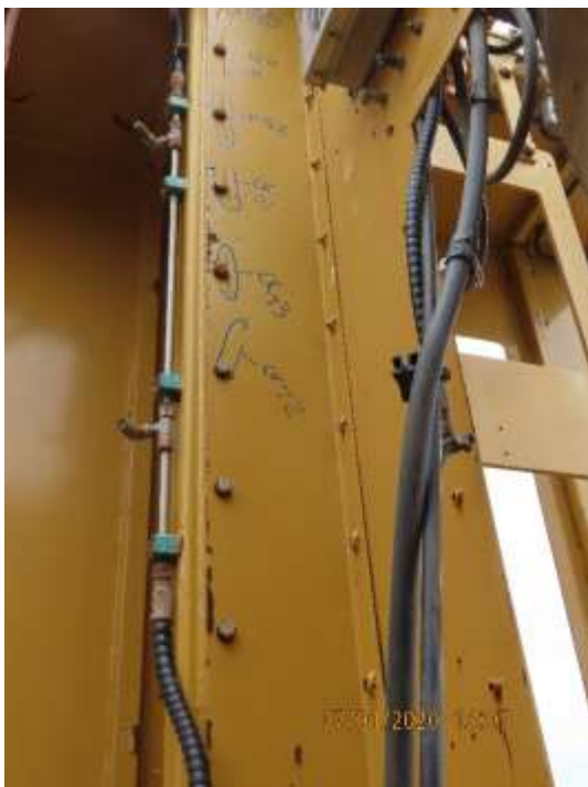
PHOTOGRAPH NO. 18 - Caterpillar 6060 excavator superstructure 200mm, 186mm, 152mm, 101mm, 93mm & 72mm cracks detected.
