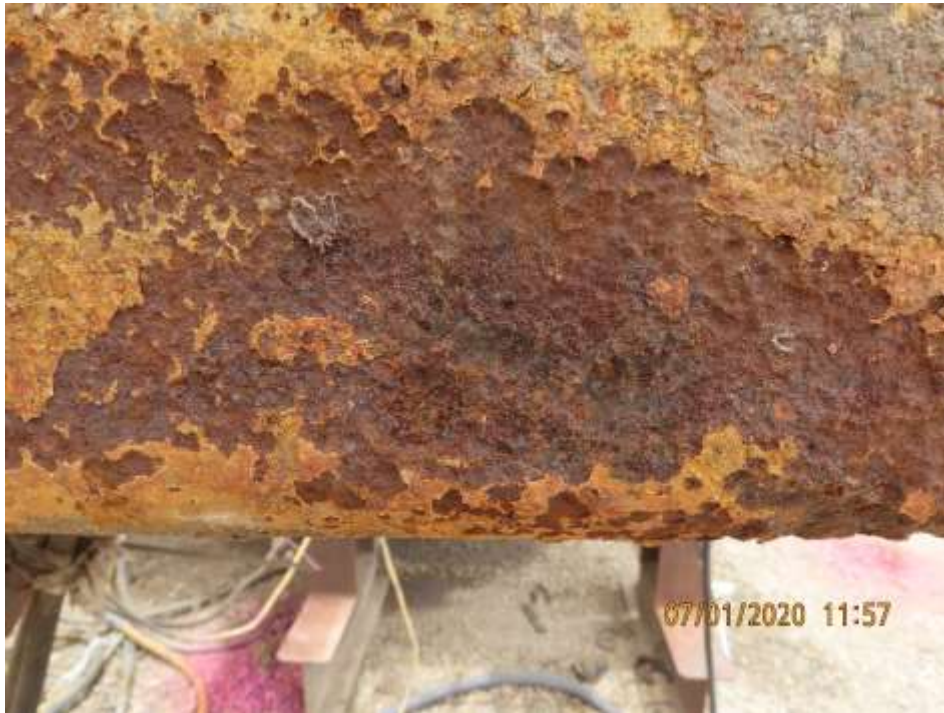
PHOTOGRAPH NO. 6 - Caterpillar 6060 excavator superstructure - corrosion detected on right hand side rail.
