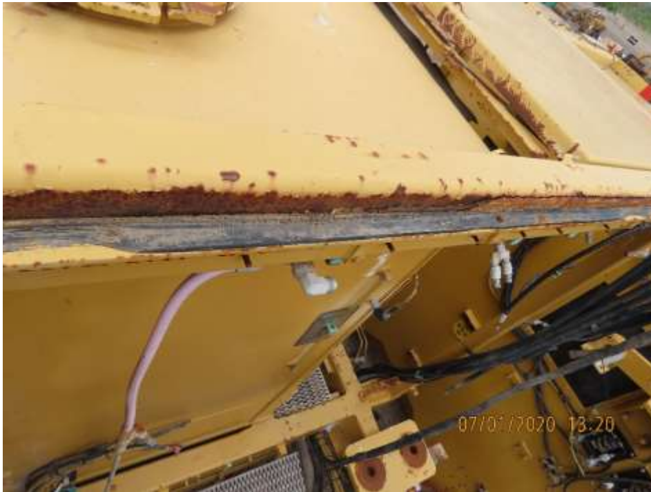
PHOTOGRAPH NO. 12 - Caterpillar 6060 excavator superstructure - 80mm crack detected.
