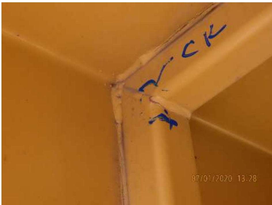
PHOTOGRAPH NO. 22 - Caterpillar 6060 excavator superstructure - crack detected on roof support.
